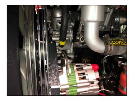
The other end of the YELLOW-marked hose attaches to the water inlet of the engine utilizing the hose barb installed in the water pump. Use (1) SAE #10 hose clamp to secure the connection.
