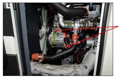
Loosen the engine alternator mounting bolts and rotate alternator towards engine to loosen the tension on the fan belt.
