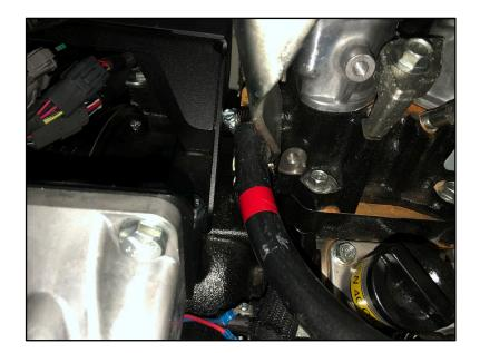
The other end of the REDmarked hose attaches to a water outlet of the engine utilizing the hose barb installed in the rear of the engine head. Use (1) SAE #10 hose clamp to secure the connection.
