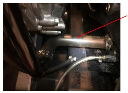
Install the larger piece of modified tubing to the radiator as shown with the stock hose clamp. Do not fully tighten yet as adjustment will be needed before final assembly.
