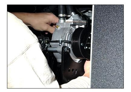
Attach the side nearest the engine using an M10x40mm bolt (920-0072-A0) and M10 NYLOC nut (920-0013-A0).
