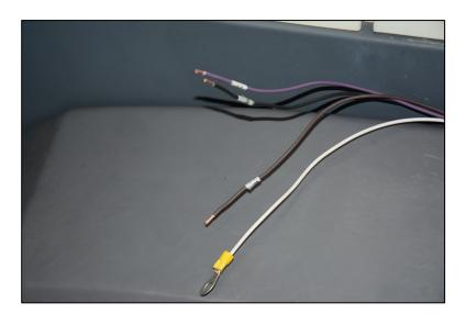
Locate the 4 voltage sensing wires. If they are terminated differently than shown, modify them to match. The purple, black, and brown wires should have approximately ¼" of insulation stripped from the ends. The white wire requires a 3/8" loop crimp terminal.
