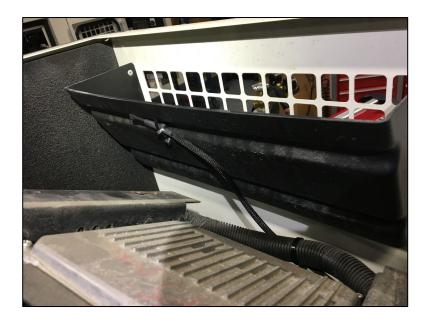
Route Outside Ambient Temperature Sensor (OATS) as shown to the rear of the generator as shown, avoiding sharp edges and hot surfaces. There may be a need to drill two small holes in the plastic baffle in order to wire tie OATS in place.
