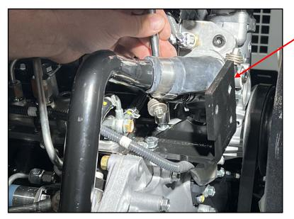
Install Mounting Bracket (140-0143-A0) using 2 M8 x 25mm bolts (920-0010-A0) and 2 M8 Flat Washers (925-0002-A0) onto machined pads on the engine as shown.
