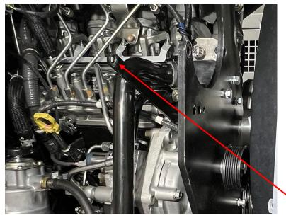
Now attach the Backing Plate to the Top Stay Weldment (140-0144-A0) using 2 M8 1.25 x 25mm bolts (920-0009-A0), 2 M8 Flat Washers (925-0002-A0) and 2 M8 1.25 NYLOC nuts (920-0031-A0).
