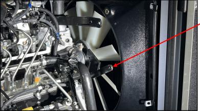
Special note: The Support Bracket (14-0461-B0) will be eliminated and replaced by a longer LHG bolt spacer in later versions of the 0130A and 0130B kits. Install the Support Bracket (14-0461-B0) using 1 M8 1.25 x 20 HEX HD Bolts (920-0009-A0), 1 M8 Lock Washer (925-0012-A0), and 1 M8 Flat Washers (925-0002-A0).
