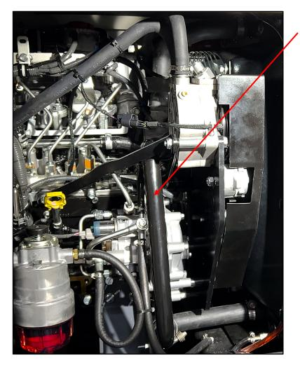
Install the formed metal tube (14-0475-A0) between the two lengths of hoses installed in previous steps using hose clamps to secure the tube to the hosing. Once placement is satisfactory, tighten all hose clamps.
