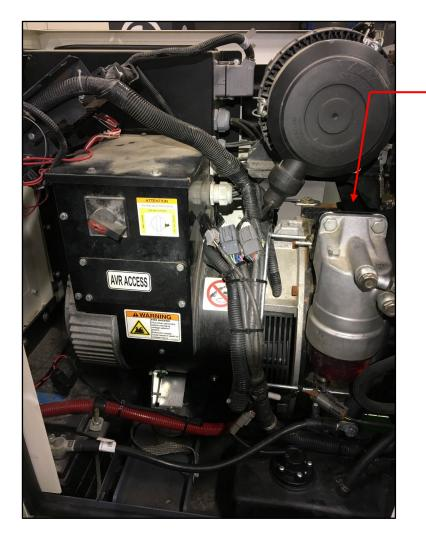
Remove the 3 bolts holding air cleaner bracket to engine bell housing (beneath air cleaner). Shift air cleaner assembly rearward to gain access to vacant port on rear of engine head.
