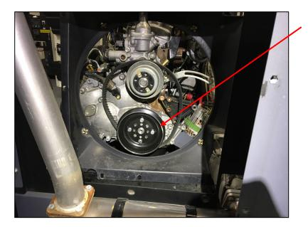
Install the Ventech supplied drive pulley (14-0421-A0) and pulley adapter (14-0435-A0) to the front of the crank pulley using 4 M8x20mm bolts (920-0009-A0) and 4 M8 lock washers (925-0012-A0).
