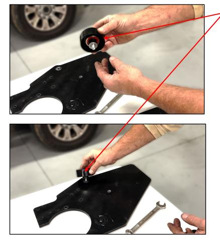
Install the Idler Pulley (981-0005-A0), with Idler Pulley Spacer (14-0456-C0) and M10 Washer (925-0031-A0) to the Backing Plate (14-0453-G0), using Hex HD Bolt (920-0019-A0).
