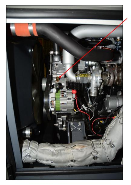
Remove 3/8" NPT plug from water pump inlet and install 3/8" NPT(M) to 5/8" hose barb (990-0135-A0) into water pump inlet using Teflon tape on the threads.
