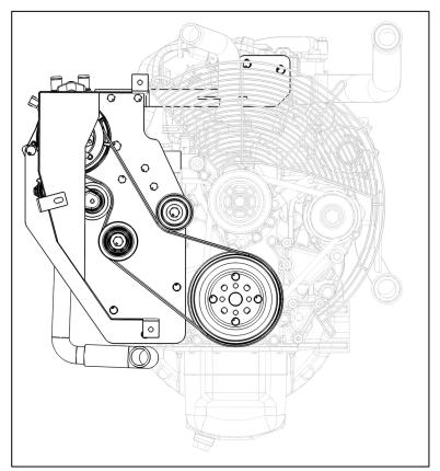
Install Belt (980-0072-A0), routing as shown in the diagram to the left.
