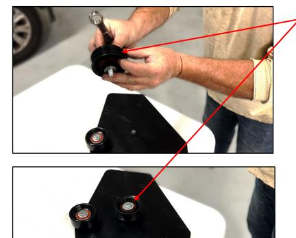
Install the Idler Pulley (981-0018-A0), with Idler Pulley Spacer (14-0456-C0) and M10 Washer (925-0031-A0) to the Backing Plate (14-0453-G0), using Hex HD Bolt (920-0019-A0).
