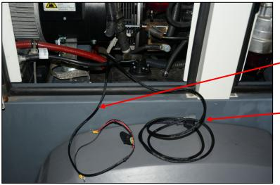
Here, the cover and grommet is shown installed. The three harness legs running out are as follows:
