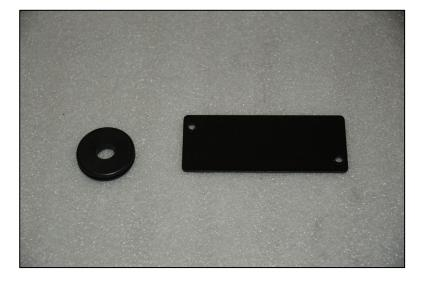
On the lower left side of the electrical cabinet, there is a small rectangular cover bolted on shown on the right here. Remove this cover and punch a 1.25" hole in it (a 3/4" conduit punch works well) to fit the grommet shown here on the left. If the cabinet does not have this cover, you will have place this hole into the box itself.
