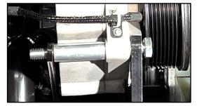
Install LHG700 into bracket assembly as shown.
