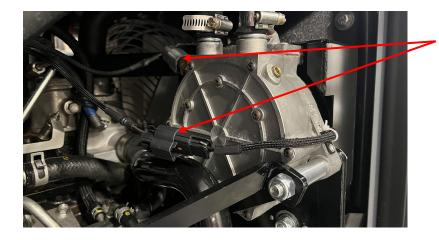
Connect LHG harness to LHG as shown. Use wire ties as needed to neatly route harness. Connectors are specific to mating connector (cannot be connected incorrectly)
