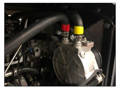
Connect two pieces of 5/8" heater hose to the LHG. The longer section is marked with RED and is the inlet to the LHG. The YELLOW marked hose is the shorter length and is the outlet from the LHG. Use (2) SAE #10 hose clamps to secure the connection.
