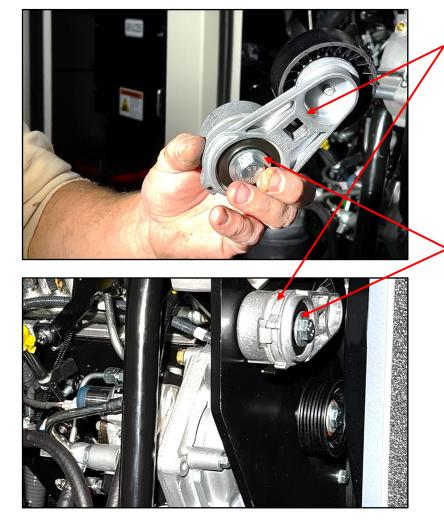
Attach the Belt Tensioner (982-0003-A0) using the M10 1.5 x 75mm bolt (920-0152-A0), oversized M10 washer (925-0031-A0), and M10 NYLOC nut (920-0013-A0)
