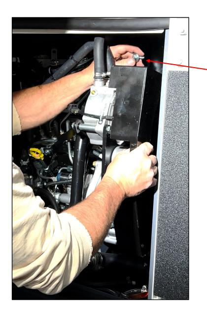
Install the LHG belt guard assembly (140-0146-A0 for 45kW, 140-0147-A0 for 25kW).
