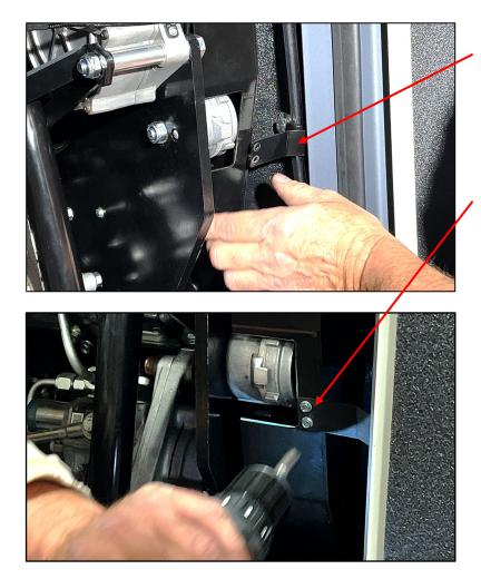
Install the LHG Belt Guard Tie Bracket (14-0549-D0) behind the hose and P-Clamp, as shown here.
