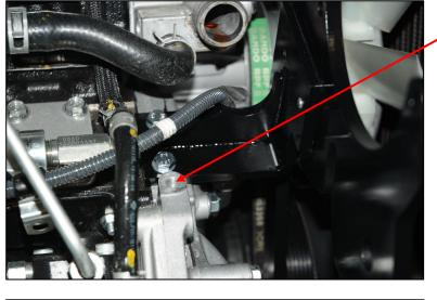
Locate the mounting boss (right side of engine) from step 4.1.2.6.
