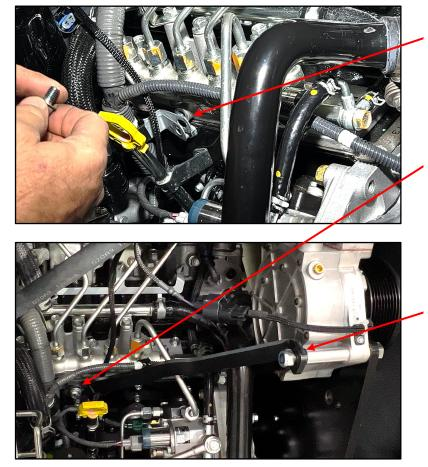
Remove the bolt holding the P-clip under the fuel lines on the left (LHG) side of the engine.
