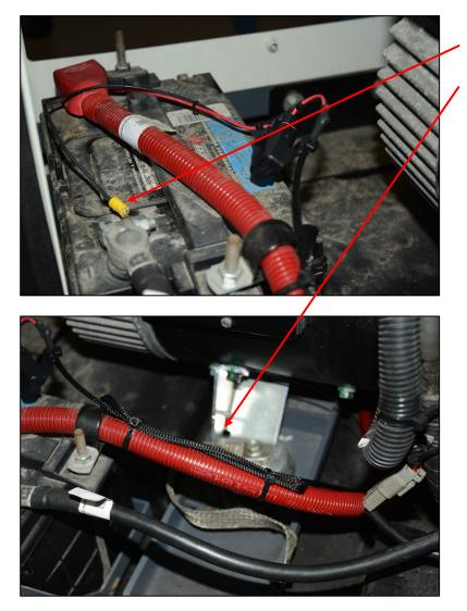
Connect battery voltage harness as shown. Use wire ties to neatly route wiring.
