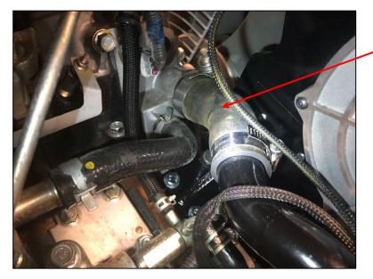
Install the shorter piece of tubing to the engine coolant intake as shown with the stock hose clamp. Do not fully tighten yet as adjustment will be needed before final assembly.
