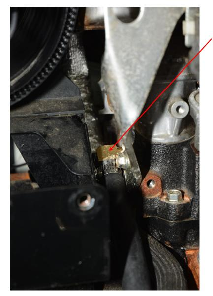
Remove 3/8" NPT plug from head and install 3/8" NPT(M) to 5/8" hose barb elbow (990-0115-A0) into head using Teflon tape on the threads.
