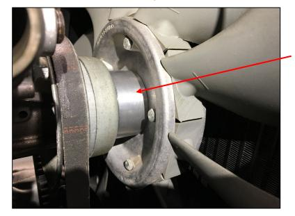
Reinstall fan keeping the original spacer and adding the additional fan spacer (14-0467-B0) and 4 M6x55mm bolts (920-203-A0).
