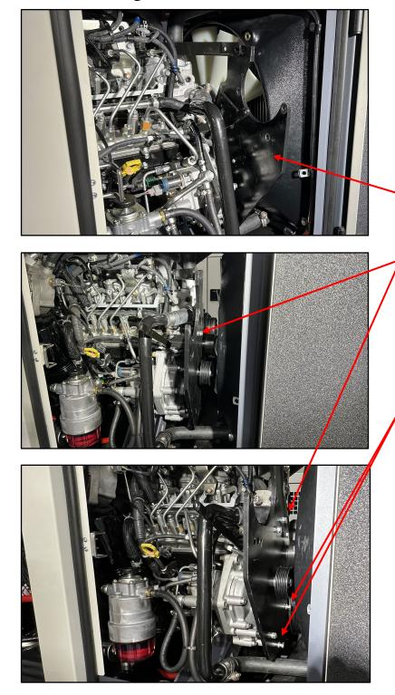
Make sure the bolts holding the Mounting Bracket (140-0143-A0) and the Support Bracket (14-0461-B0) are loose to allow for easier positioning and installation of the Backing Plate.
