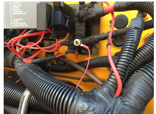
Red Harness wire connects to the Vehicle 12V Terminal Post that has a direct connection to the Positive post of the vehicle battery.
