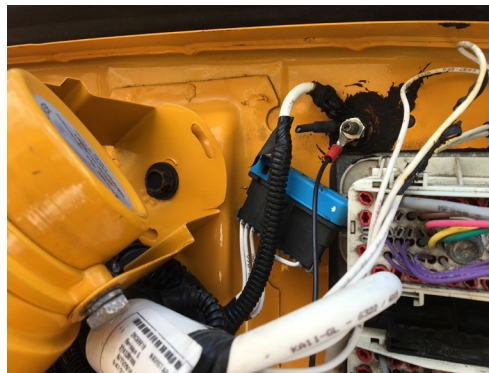
Black Harness wire connects to a Chassis Ground Terminal Post on bulkhead that has a direct connection to the Negative post of the vehicle battery.
